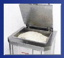
The cover automatically opens upon completion of the press cycle and a uniform block of pastry dough or fat lays on a raised plate and is ready for further processing.
