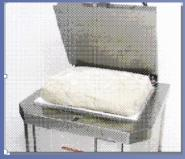
A pre-scaled amount of dough or fat portion is placed into the chamber. The press cycle starts automatically once the operator closes the lid.
