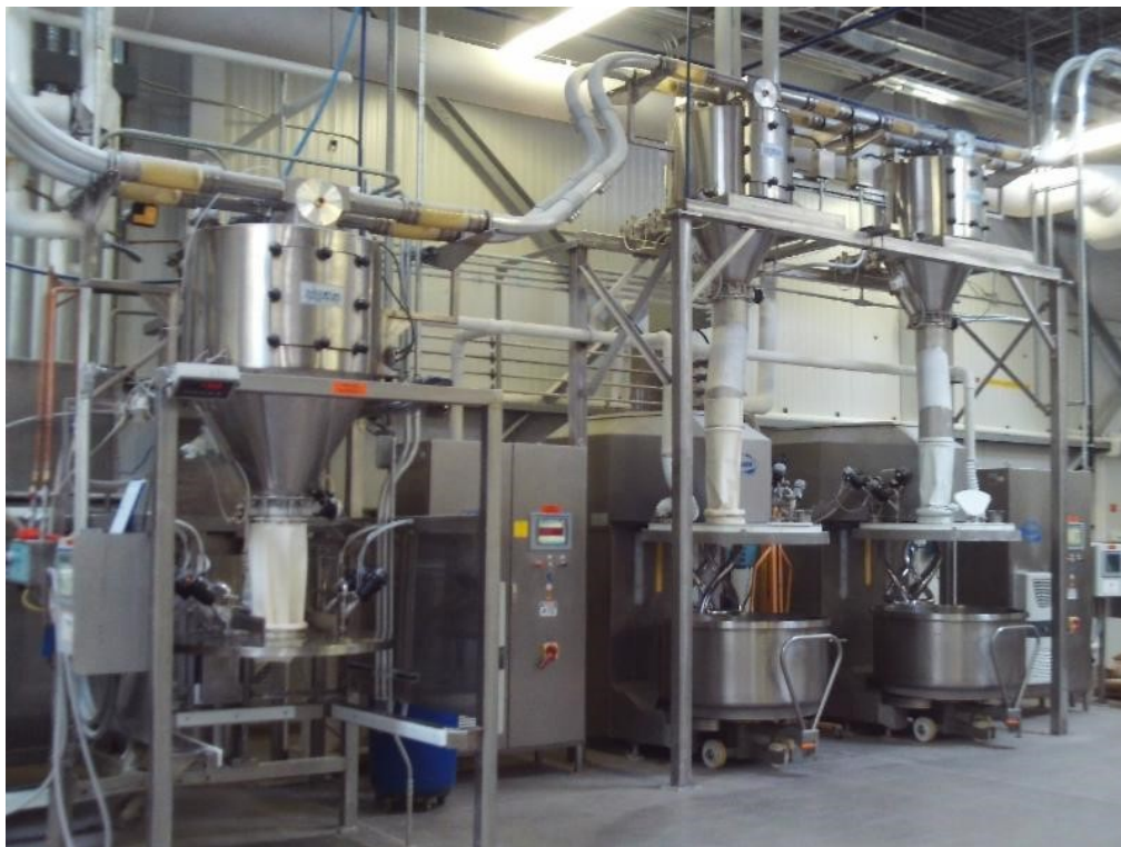
500 Pound Capacity Custom Bowl Charge Station with Liquid Ingredient Dosing. Two Weigh Hopper 'Direct to Mixer' Dispensing Station Liquid Ingredient Dosing.
