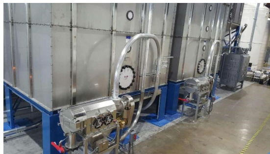
Centrifugal Sifters w/ 30-Mesh Screen and 110,000 Capacity Stainless Steel Indoor Flour Bins
