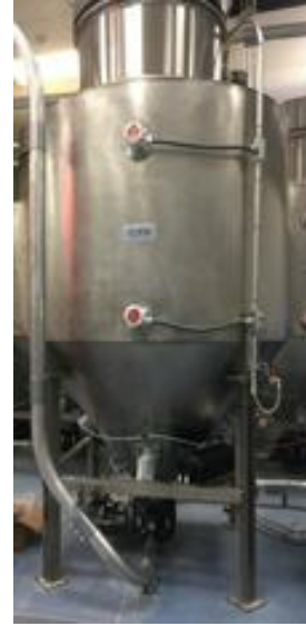
5,000 Lb Capacity Stainless Steel Ingredient Day Bin w/ Automatic High/Low Level Control
